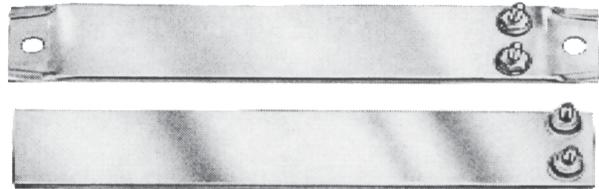
Standard Ultima® Strip Heaters are manufactured to 40W/IN<sup>2</sup> heat capacity and 240 volt rating. In this manner tandem Ultima® strips or bands can be wired to 240 or 480 volt source. These heaters can operate up to 1200°F continuous operation with one of the highest dielectric properties attainable in industrial applications today. Applications include: Film die head heating, platen and vacuum forming machinery.
